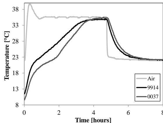
Figure 13: Temperature as a function of time of the air in the oven and the two PCM (9914 and 0037).
