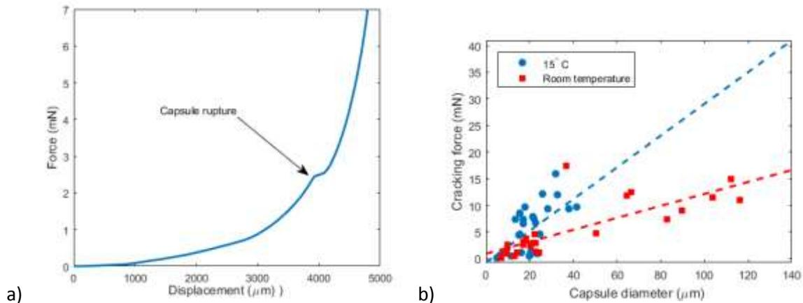
Figure 8: a) Typical force-displacement diagram for a PCM microcapsule<sup>1</sup>; b) A relationship between capsule diameter and cracking force for two tested temperature regimes.
