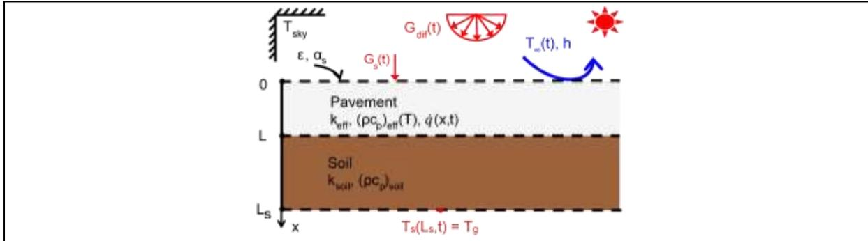
Figure 10: Schematic of the heat transfer model consisting of a pavement section of length  $L$  exposed to the ambient air and a soil section with a constant ground temperature at its bottom surface.
