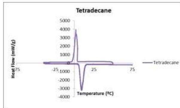
Figure 1: DSC scan of tetradecane. The endothermic part of the spectrum gives the melting temperature obtained ( $T=9.33^{\circ}\text{C}$ ) and the heat of fusion ( $\Delta H_f=183.3 \text{ J/g}$ ).
