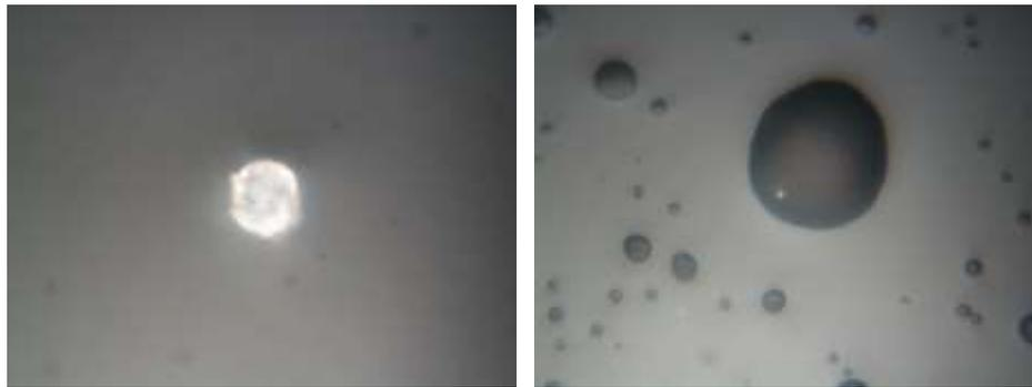
Figure 7: A single PCM microcapsule before (left) and after (right) the nanoindentation test
