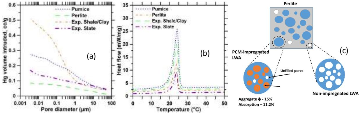
Figure 4: (a) Pore volume intruded for the different LWAs, (b) DSC scans of the different LWAs impregnated with PCMs, and (c) illustration of the mixture design method to contain 5% of PCM by volume of the mortar
