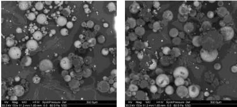
Figure 3: Scanning electron images of the product obtained in the encapsulation of paraffin wax. Different diameter size particles can be seen, some as large as  $250 \mu\text{m}$ .
