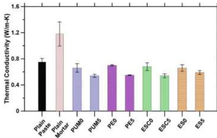
Figure 5: Thermal conductivity determined after 28 days of hydration for the paste and mortars. The first data is for OPC paste, and the rest are for mortars where the paste volume fraction is 0.50.
