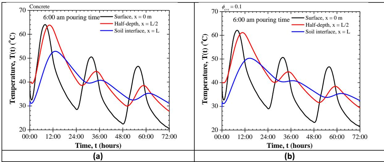
Figure 11: Transient temperature evolutions within pavement sections composed of (a) plain concrete, and (b) concrete containing PCM ( $\phi_{c+s} = 0.1$ ). The pavements were poured at 6:00 am and exposed to outdoor temperature and solar radiation corresponding to a hot September day in Los Angeles, CA.
