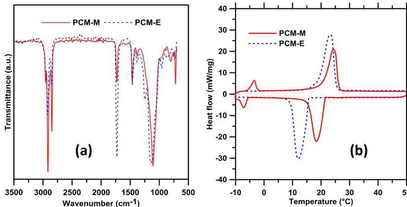
Figure 3: (a) FTIR spectra, and (b) DSC scans, of PCM-M and PCM-E. The DSC scans were carried out in the temperature range of  $-10^{\circ}\text{C}$  to  $50^{\circ}\text{C}$  at a heating rate of  $5^{\circ}\text{C}/\text{min}$ .
