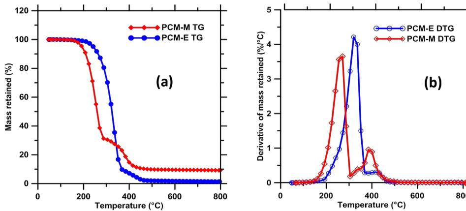
Figure 2: (a) Thermogravimetric (TG), and (b) differential TG curves of PCM-M and PCM-E.
