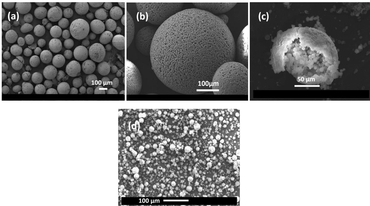
Figure 1: Micrographs of: (a) Micronal PCM, (b) and (c) Micronal PCM showing smaller capsules that are agglomerated to form the larger capsule, and (d) Encapsys PCM, which is composed of discrete particles.
